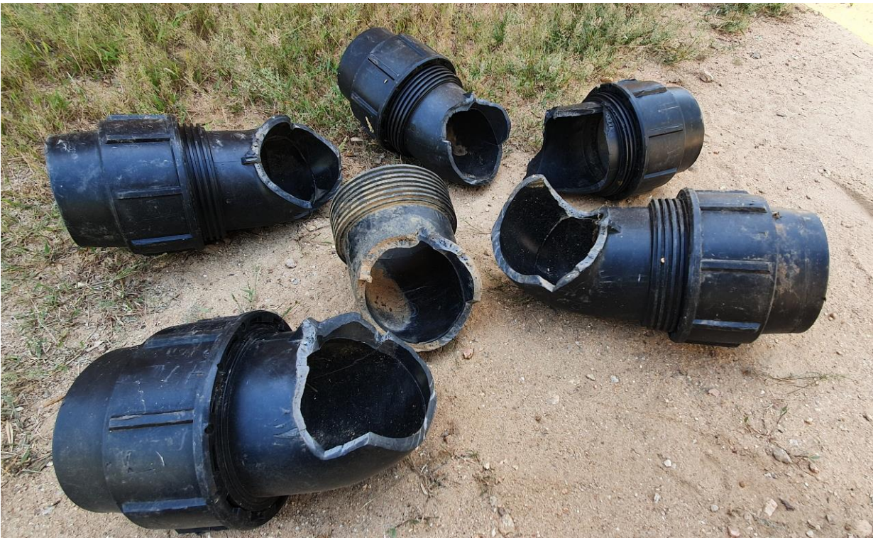
Figure 5. Broken pipe fittings in Bredjing. The pipelines crossing wadis need constant repairs.
