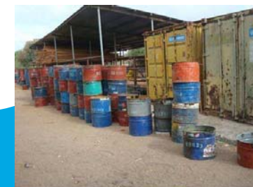
Waste bins fabricated from half cut drums awaiting distribution at Hagadera, Kenya
